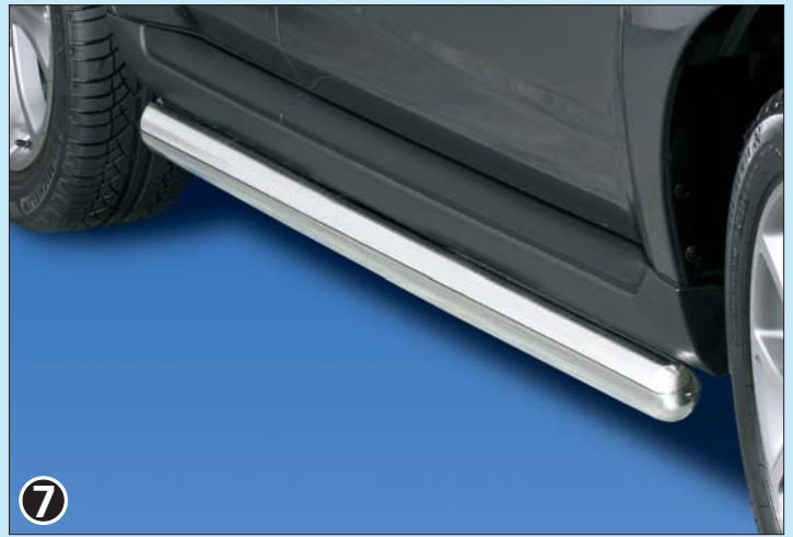
7 Side bar 70mm straight Flankenschutzrohr 70mm gerade Stainless steel / Edelstahl 12D 4051
